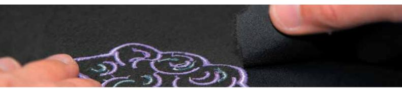
Without suitable stabilisation, the base material will pucker and form wrinkles. For smooth and distortion-free embroidery results, you should always use a suitable backing.
